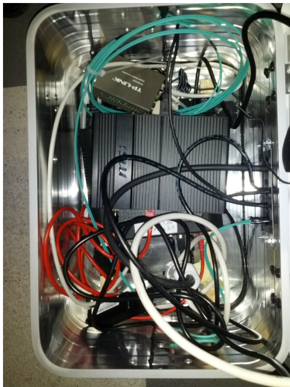
Figure 12: Components of central communication: Media converter for fiber line, PC running server software, PoE enabled switch
