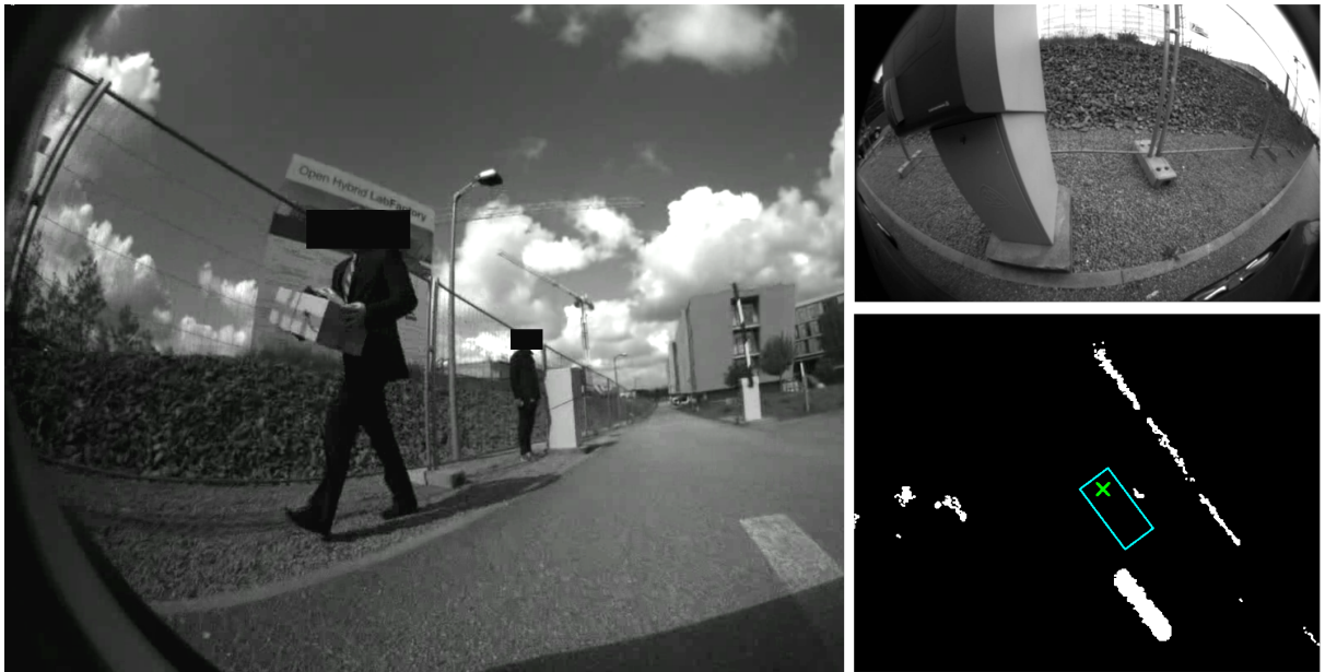
Figure 9: Moving pedestrians in close vicinity to the ego vehicle (left) and small perception noise when passing narrow gates (right) were often the cause when no valid solution trajectory could be computed by the local motion planner.
