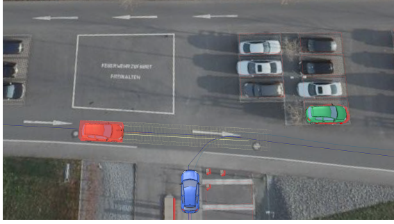
(6.a) The ego vehicle (blue) waits at the intersection since the oncoming vehicle from the left (red = relevant object at the intersection) matches all conditions, including the check for the incoming lane.
