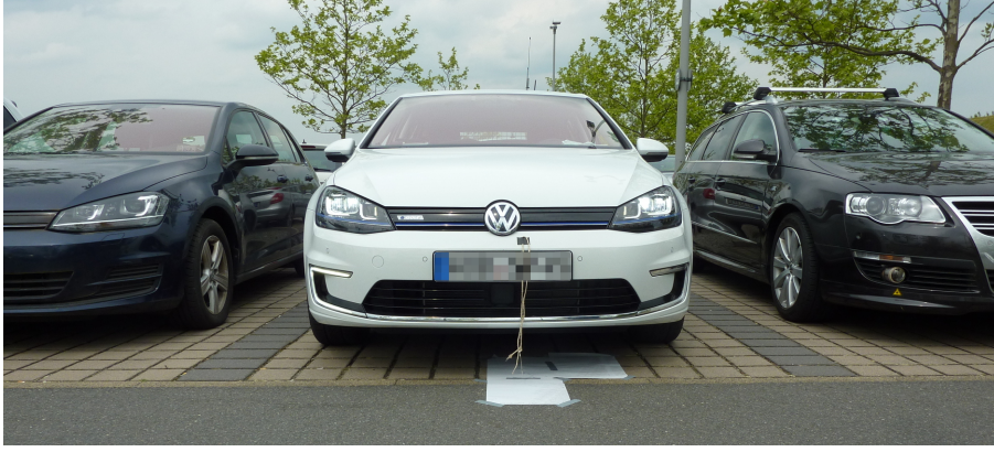
Figure 22: Manual recording of the final vehicle pose inside the parking spot via a plumb line attached at the vehicle's front.
