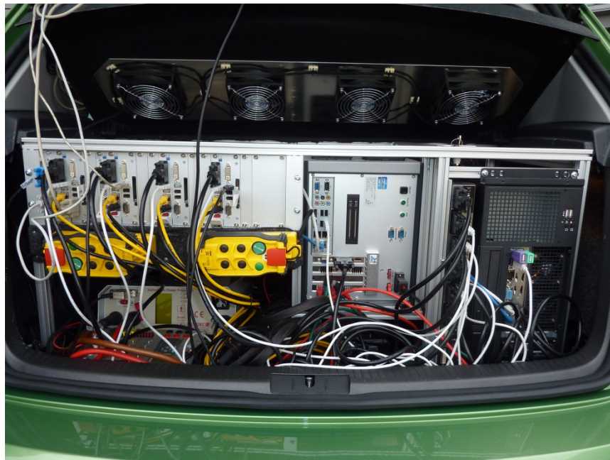
Figure 12: Computing system installed in vehicle trunk, 6 Rack PCs, two separated computing systems for mono and stereo processing
