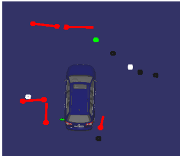
Figure 31: Line and Point Objects triangulated immediately in the Ultrasonic ECU
