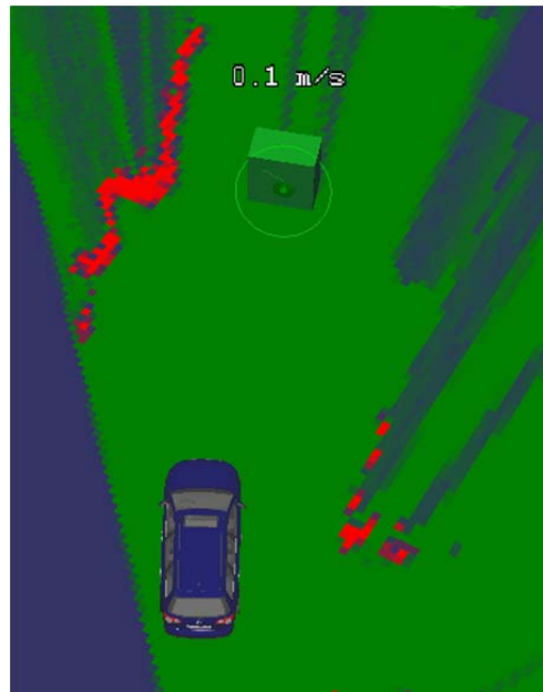
Figure 34: Driving Layer with Overlay Bound Box resulting from Object Fusion module already labeled dynamic e.g. by the image-based object detection and classification
