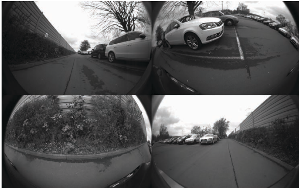
Figure 1.2: Images from the four fisheye cameras (front, right, left, rear)
