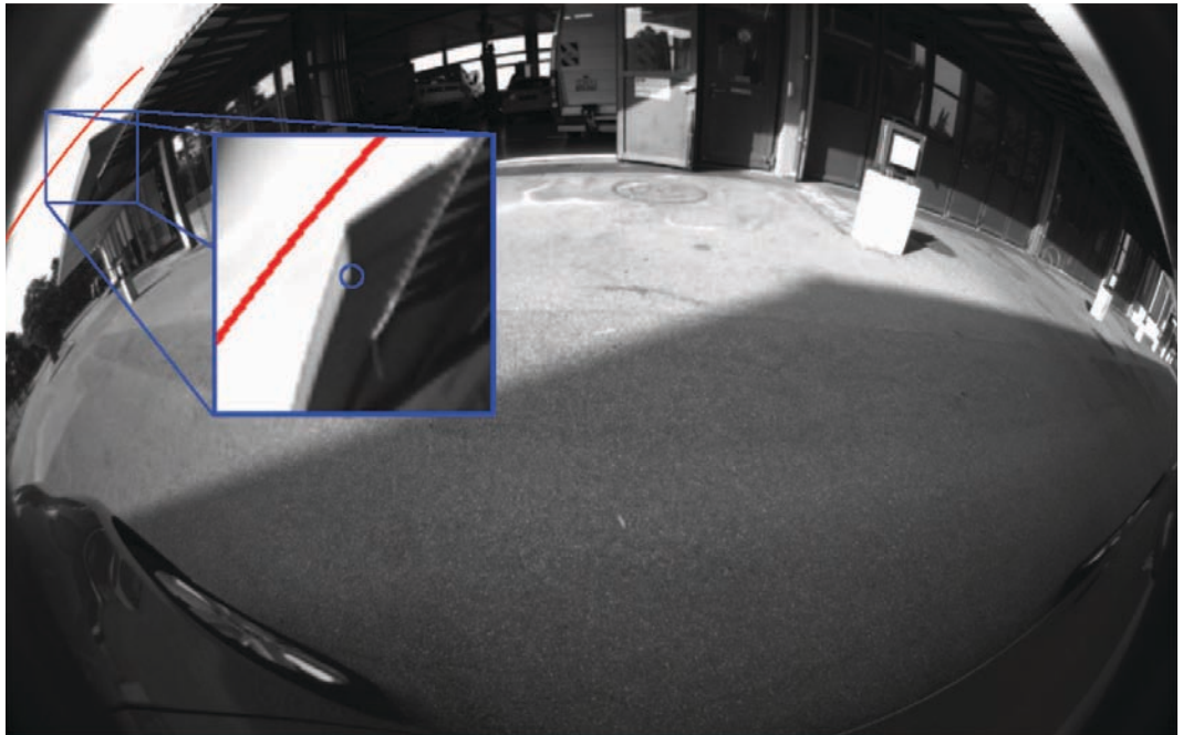
(b) Right camera image with epipolar line (red) and hand-picked reference point (blue)
