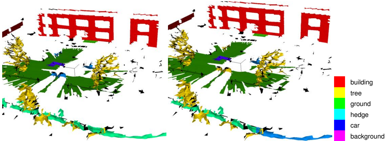
Figure 1: Semantic labeling using laser data. In this example, a car par was scanned by a rotating laser scanner and a classifier was trained on 6 different classes. The left figure shows the ground truth labeling, and the right one shows the classification result.
