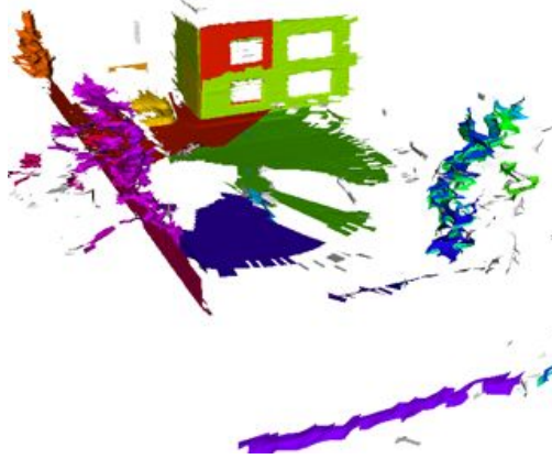
Figure 3: Mesh segmentation. Every segment has a different color assigned. In this example, the mesh has self-overlapping parts, which is why e.g. the building is split into several segments. Note that “rough” surfaces such as those on the trees are segmented as well as smoother regions such as the ground.
